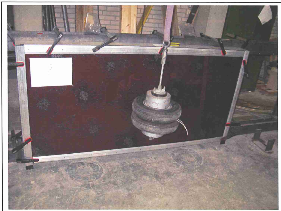
Fig. 10 Test / glass pane 2
