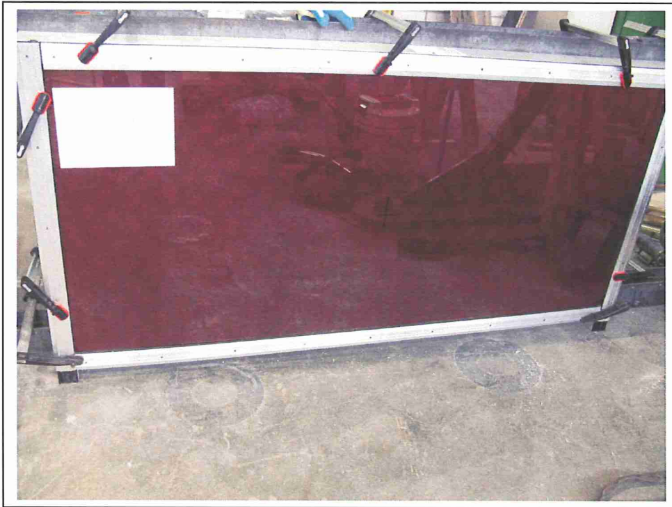
Fig. 19 Glass pane 6 prior to the impact test
