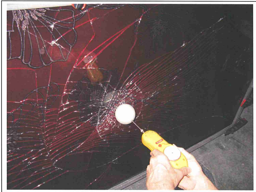
Fig. 5 Test using the ball \varnothing 76 mm
