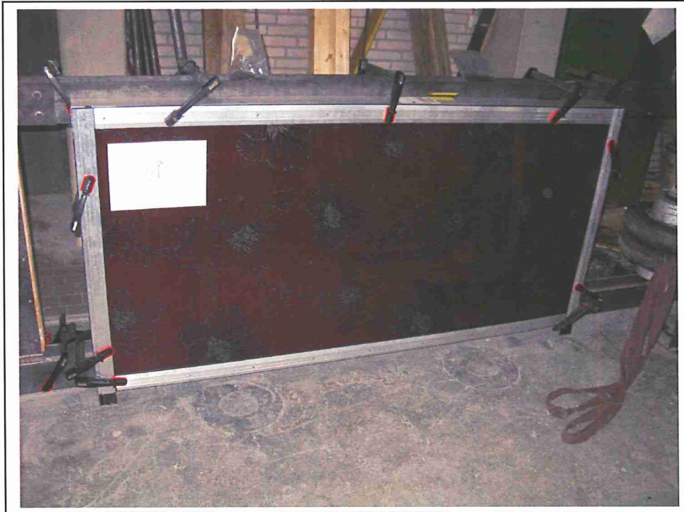
Fig. 1 Test frame / glass pane 1
